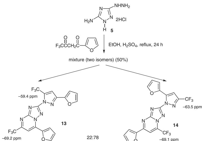
**Scheme 5** Synthesis of asymmetrically fluorinated pyrazolo-1,2,4-triazolo-pyrimidines
