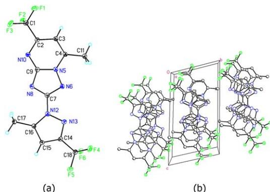
**Figure 2** (a) Molecular structure of **9** (30% thermal displacement) showing the numbering scheme. Hydrogen atoms are shown (arbitrary spheres) but are unlabelled for clarity. (b) Packing diagram of **9** (ball and stick) viewed down the *a*-axis, showing the alternating stacks. Hydrogen atoms have been omitted for clarity.
