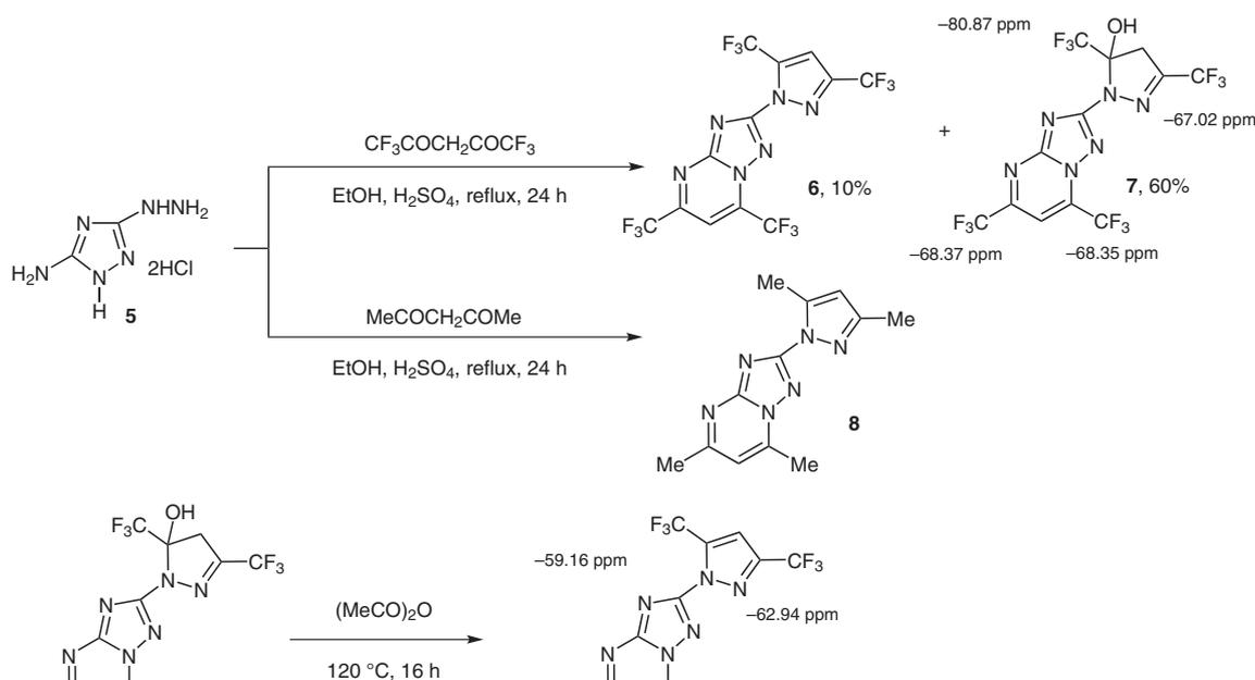
Scheme 3 Cyclization reactions of 5-amino-3-hydrazino-1,2,4-triazole
