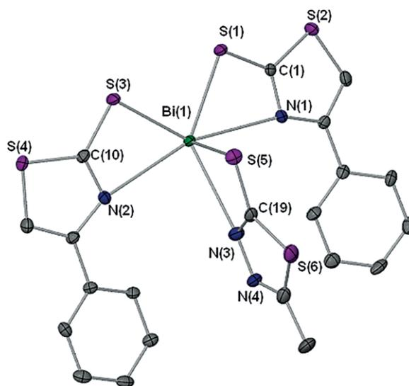
Figure 5. Asymmetric unit of [Bi(MBT)<sub>2</sub>(5-MMTD)] **3** with thermal ellipsoids shown at 50 % probability. Hydrogen atoms have been omitted for clarity.
