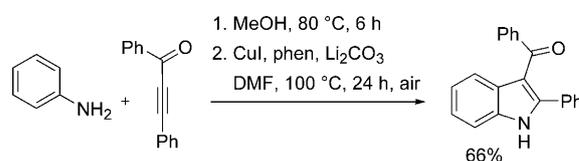
**Scheme 2.** Synthesis of indoles from anilines and  $\alpha,\beta$ -ynones omitting the isolation of enaminone intermediates.
