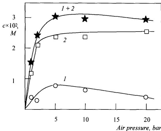
**Figure 1.** Oxidation of cyclohexane (0.46 M) at 40 °C with  $H_2O_2$  (0.2 M) catalyzed by  $VO_3^-$  – PCA in autoclave (total volume 100 mL; volume of the solution 10 mL). Dependences of concentrations of cyclohexanone (1), cyclohexanol (2) and their sum (1 + 2) after 1 h on the air pressure are shown.
