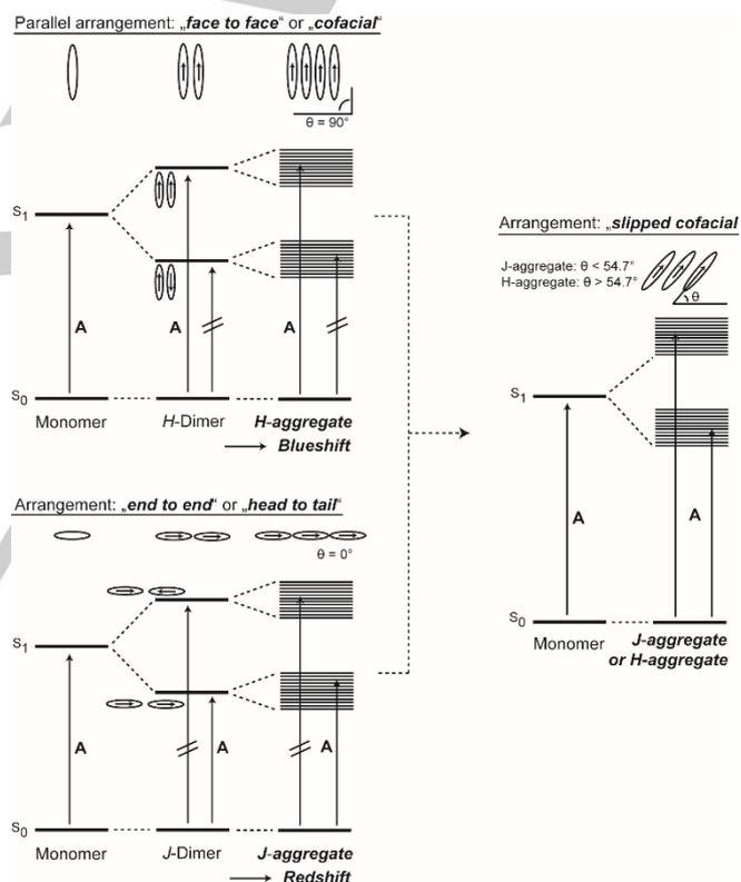
**Figure 1.** Schematic representation of the photophysical absorption properties (A) of a *J*- or *H*- aggregate. Slipped facial aggregates are tilted aggregates. In this case it depends on the staggering angle of which aggregation type is formed.
