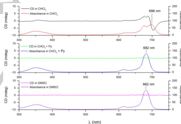
**Figure 5.** CD and absorbance spectra of **2** measured in chloroform, chloroform with pyridine and in DMSO.
