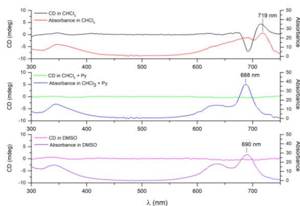
**Figure 6.** CD and absorbance spectra of **4** measured in chloroform, chloroform with pyridine and in DMSO.
