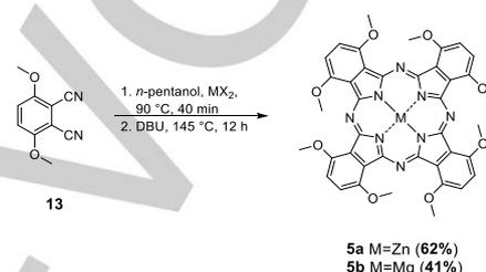
**Scheme 6.** Synthesis of **5a** and **5b** from dimethyl 3,6-dimethoxyphthalonitrile.
