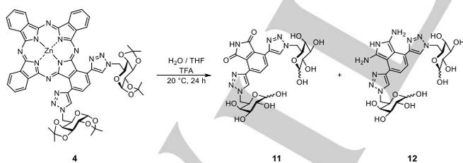
**Scheme 4.** Deprotection of the isopropylidene groups lead to detetramerization of the phthalocyanine core. Phthalimid **11** and diiminoisindole **12** were formed.
