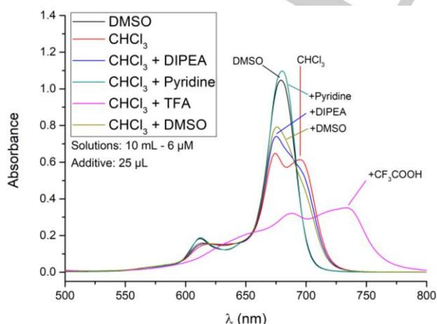
**Figure 2.** UV/Vis spectra (Q band) of **2** measured in different solvents.
