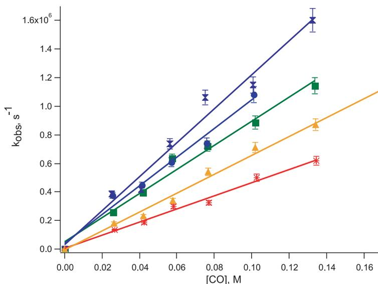
Fig. 3. Plots of  $k_{\text{obs}}$  vs.  $[\text{CO}]$  for the decay of the transient  $\text{Mo}(\text{CO})_5(\text{Sol})$  as monitored at  $1931\text{ cm}^{-1}$  in cyclohexane solution.
