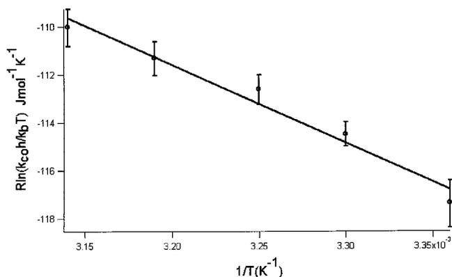
Fig. 4. Eyring plot of  $k_{\text{CO}}$  data in Fig. 3 for the reaction of CO with  $\text{Mo}(\text{CO})_5(\text{Sol})$  in cyclohexane solution.
