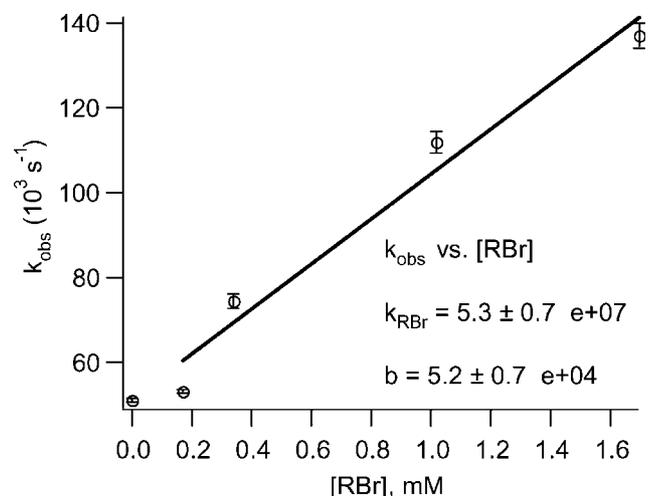
Fig. 1. Plot of  $k_{\text{obs}}$  vs.  $[\text{RBr}]$  for the decay of transient,  $\text{Mo}(\text{CO})_5(\text{Sol})$  in 298 K cyclohexane under  $P_{\text{CO}} = 1.0$  atm.
