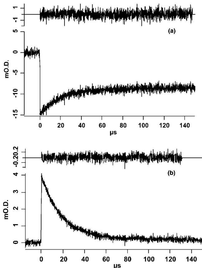
Fig. 2. Temporal absorbance changes at IR frequencies characteristic of (a)  $\text{Mo}(\text{CO})_6$  ( $1987\text{ cm}^{-1}$ ) and of (b)  $\text{Mo}(\text{CO})_5(\text{Sol})$  ( $1931\text{ cm}^{-1}$ ) subsequent to 308 nm flash photolysis of  $\text{Mo}(\text{CO})_6$  in cyclohexane solution.  $T = 298\text{ K}$ ,  $P_{\text{CO}} = 1.0$  atm.
