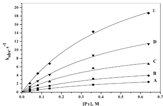
**Fig. 4** Plots of  $k_{\text{obs}}$  vs. [pyridine] for the reaction with  $1 \times 10^{-3}$  M *trans*-[(CH<sub>2</sub>Cl)Co(Hdmg)<sub>2</sub>H<sub>2</sub>O] as a function of temperature. Experimental conditions: pH = 8,  $I = 0.1$  M, and temperature 20 (A), 25 (B), 30 (C), 35 (D) and 40 (E) °C.
