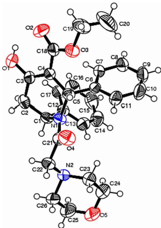
**Figure 2.** ORTEP plot of **9**. The important bond lengths (Å): C(1)–N(1) = 1.470(3); C(5)–N(1) = 1.476(3); C(21)–N(1) = 1.356(3); C(21)–O(4) = 1.218(3); C(21)–C(22) = 1.520(3); C(2)–C(3) = 1.484(3); C(3)–C(4) = 1.346(3); C(4)–C(5) = 1.507(3). The important bond angles (°): N(2)–C(22)–C(21) = 114.4(19); O(4)–C(21)–N(1) = 121.4(2); N(1)–C(21)–C(22) = 120.2(2); N(1)–C(5)–C(6) = 113.3(18); C(1)–N(1)–C(5) = 116.8(17); C(21)–N(1)–C(5) = 117.1(19); C(21)–N(1)–C(1) = 123.9(18).
