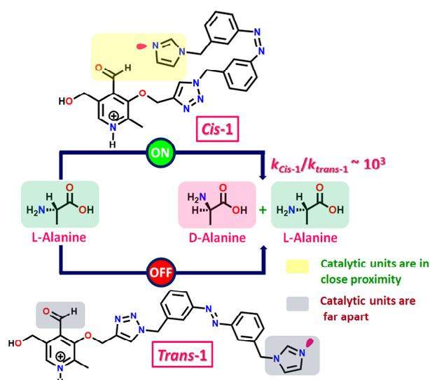
**Figure 3.** Photoregulation of L-Ala to D-Ala transformation with the PLP-azobenzene-imidazole triad **1**.
