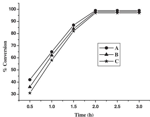
Fig. 3. Catalytic transfer hydrogenation of: (A) Acetophenone, (B) benzophenone, (C) cyclohexanone in different time intervals.
