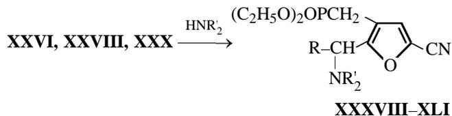
$\text{R} = \text{CH}_3$ ,  $\text{R}'_2 = (\text{CH}_2)_2\text{O}(\text{CH}_2)_2$  (**XXXVIII**);  $\text{R} = \text{CH}_3$ ,  $\text{R}'_2 = \text{C}_2\text{H}_5$  (**XXXIX**);  $\text{R} = \text{C}_2\text{H}_5$ ,  $\text{R}'_2 = (\text{CH}_2)_5$  (**XL**);  $\text{R} = (\text{CH}_3)_2\text{CH}$ ,  $\text{R}'_2 = (\text{CH}_2)_5$  (**XLI**).
