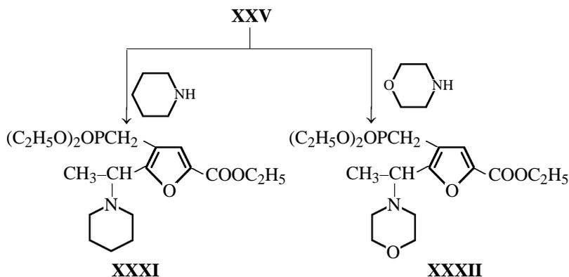
Amino phosphonates **XXXI** and **XXXII** are yellow-brown oils. Their  $^1H$  NMR spectra contained the signals of the CH-N fragment at the furan ring at  $\delta$  3.84 and 3.75 ppm, respectively. The methylene group at phosphorus in both cases gave two doublets with the constant  $J_{HP}$  20 Hz (3.02 and 3.08 ppm for **XXXI**, and 2.88 and 2.91 ppm for **XXXII**).
