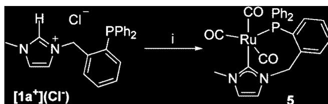
**Scheme 4.** Two step synthesis of the ruthenium(0) complex **5** starting from  $[\mathbf{1a}^+](\text{Cl}^-)$ : i) 1 equiv. of KHMDS, 0.33 equiv. of  $\text{Ru}_3(\text{CO})_{12}$ , tetrahydrofuran, r.t., 20 h.
