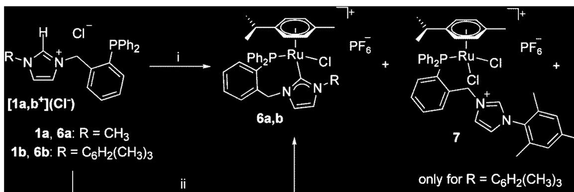
**Scheme 5.** Synthesis of the ruthenium(II) NHC complexes **6a,b** and **7**. i) 0.55 equiv. of  $\text{Ag}_2\text{O}$ ,  $\text{CH}_2\text{Cl}_2$ , 18 h, r.t., 0.45 equiv.  $[(\eta^6\text{-cymene})\text{RuCl}_2]_2$ , 18 h, r.t., 2 equiv. of  $\text{KPF}_6$ , 24 h, r.t.; ii)
