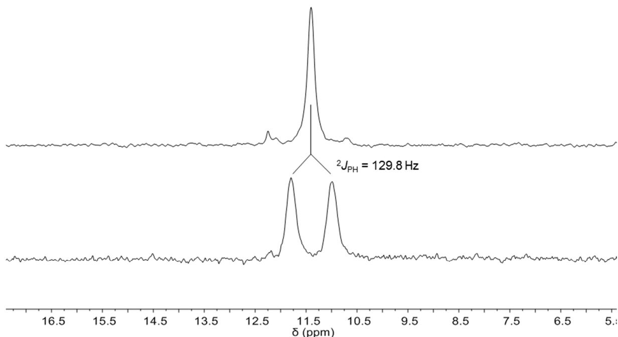
**Figure 3.** The de-coupled (top) and coupled  $^{31}\text{P}$  NMR spectrum (bottom) of compound **4** measured in  $\text{CD}_2\text{Cl}_2$  solution.
