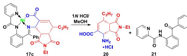
**Scheme 3** Disassembling of nickel(II) complex **17c** to release target  $\beta$ -amino acid **20** and recovery of the ligand **21**
