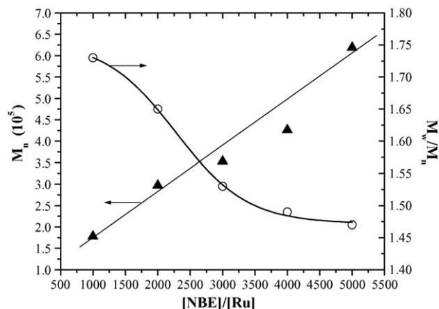
Fig. 1. Values of  $M_n$  and  $M_w/M_n$  recorded by GPC during the ROMP of norbornene as a function of [NBE]/[Ru] molar ratio using  $[\text{RuCl}_2(\text{PPh}_3)_2(\text{NH}_2^t\text{Bu})_2]$  in  $\text{CHCl}_3$  at RT; [Ru] = 1  $\mu\text{mol}$ , 5  $\mu\text{L}$  of EDA.
