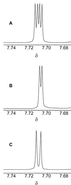
Fig. 3 The signal of the proton in the 4-position of the thiazole ring observed in the  $^1\text{H}$  NMR spectrum of **20b** (A); after selective homonuclear proton decoupling (B), and after selective heteronuclear phosphorus decoupling (C).
