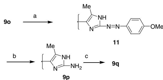
**Scheme 2.** Reagents and conditions: (a) 4-methoxybenzenediazonium tetrafluoroborate; (b) H<sub>2</sub>/PtO<sub>2</sub>/ethanol; (c) Ac<sub>2</sub>O/Py.
