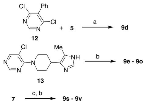
**Scheme 3.** Reagents and conditions: (a) K<sub>2</sub>CO<sub>3</sub>/diglyme/150 °C; (b) arylboronic acids/Pd(Ph<sub>3</sub>P)<sub>4</sub>/Na<sub>2</sub>CO<sub>3</sub>/DMF/80 °C; (c) NaOMe or NaO<sup>*i*</sup>Pr or morpholine.
