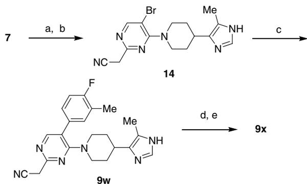
**Scheme 4.** Reagents and conditions: (a) *tert*-butyl cyanoacetate/NaH/THF/heat/2 days; (b) TFA/60 °C; (c) 4-fluoro-3-methylphenylboronic acid/Pd(Ph<sub>3</sub>P)<sub>4</sub>/Na<sub>2</sub>CO<sub>3</sub>/DMF/80 °C; (d) NaOH/MeOH; (e) isopropylamine/carbonyldiimidazole/triethylamine.
