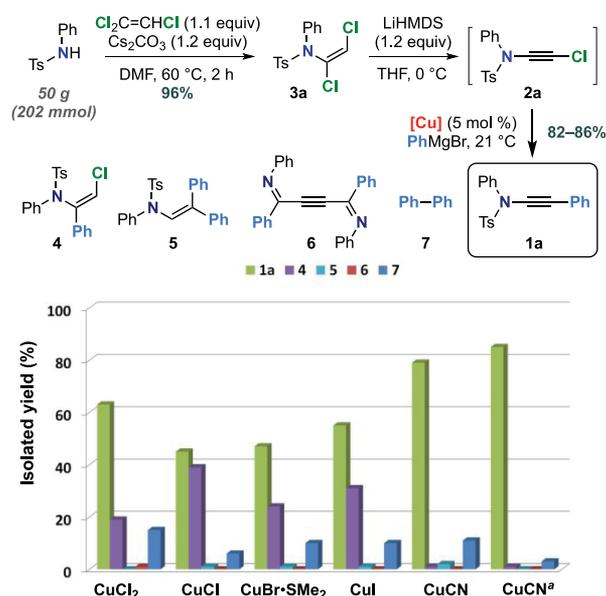
**Figure 2.** Optimization of the conversion of dichloroenamide 3a to ynamide 1a. <sup>a</sup> Optimized conditions: PhMgBr (1.03 equiv), [CuCN·2P(OMe)<sub>3</sub>] (1.25 mol %), TBME (0.34 M), 21 °C, 10 min, 82–86%.
