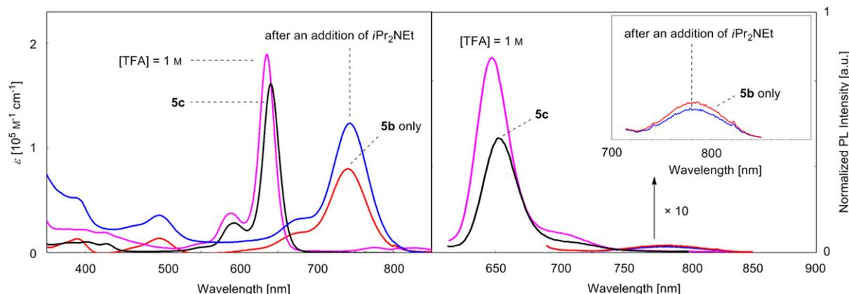
Fig. 4. The absorption spectra (left) and the emission spectra (right) of **5b** after an addition of *i*-Pr<sub>2</sub>NEt.
