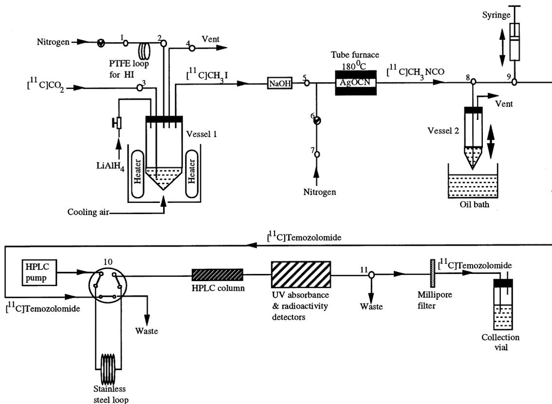
**Figure 2.** Automated system for the radiosynthesis of [3-*N*-<sup>11</sup>C-methyl]temozolomide (**9**) from [<sup>11</sup>C]iodomethane (**12**) via [<sup>11</sup>C-methyl]methyl isocyanate (**8**).
