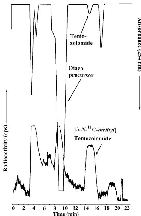
**Figure 3.** A typical HPLC profile from the radiosynthesis of [3-*N*-<sup>11</sup>C-*methyl*]temozolomide (**9**).
