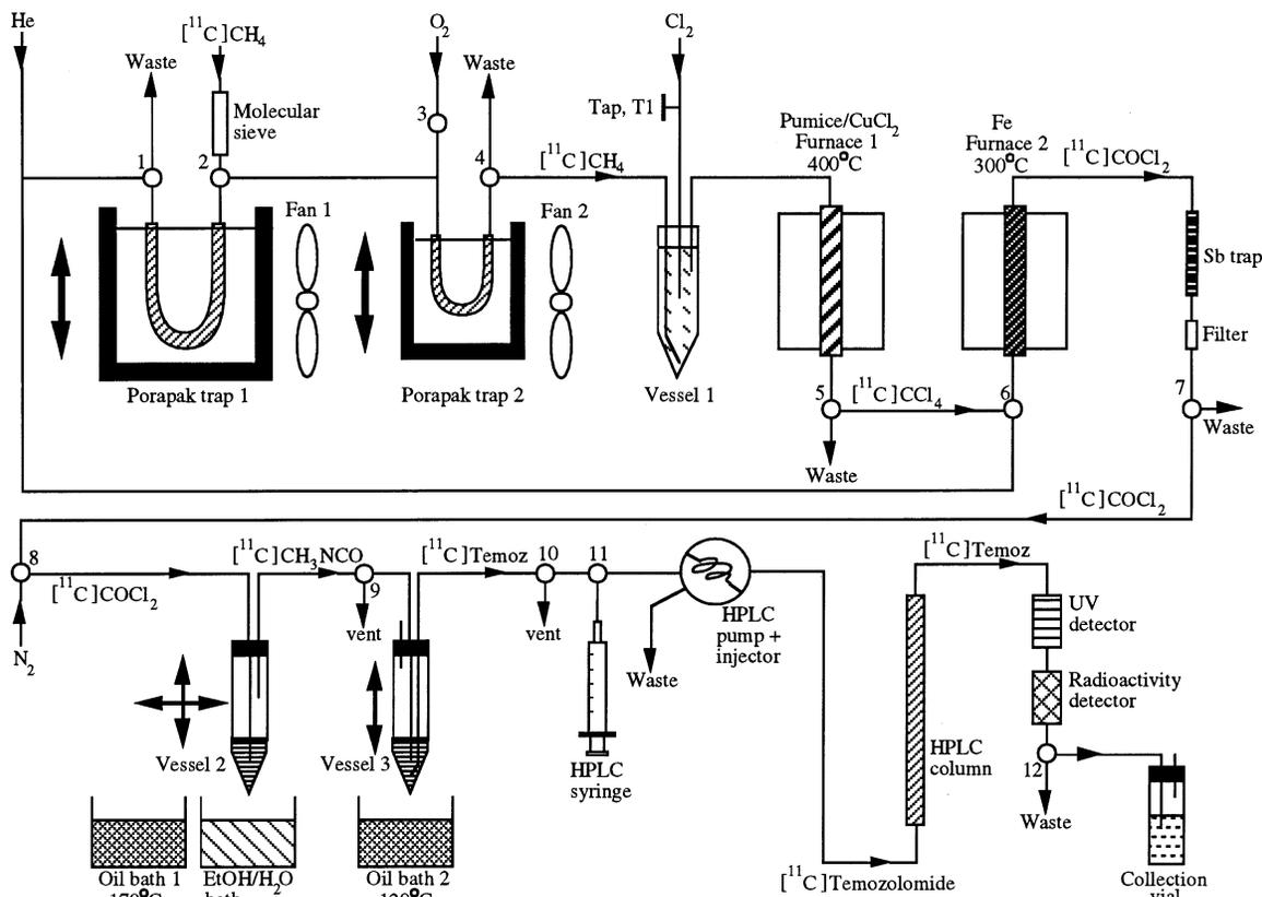
**Figure 5.** Automated system for the radiosynthesis of [4- $^{11}\text{C}$ -carbonyl]temozolomide (**11**) from [ $^{11}\text{C}$ ]phosgene (**6**) via [ $^{11}\text{C}$ -carbonyl]-methyl isocyanate (**10**).
