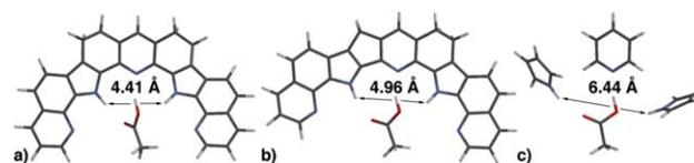
**Figure 3.** Comparison of acetic acid complexes derived from (a) **1**, (b) model receptor **1-pent**, and (c) their ‘free floating’ donor–acceptor fragments. As the  $\text{DH}\cdots\text{HD}$  distance increases (from (a) to (c)), the  $\text{O}-\text{C}=\text{O}$  unit of the guest becomes more nearly coplanar with the D-‘Sp’-D atoms.
