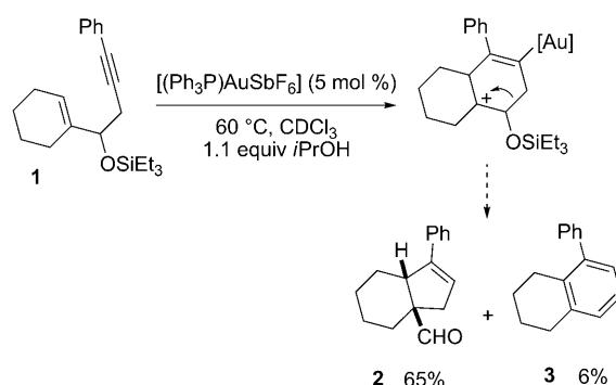
**Scheme 1.** Gold-catalyzed cyclization/pinacol rearrangement and the competing reaction according to Kirsch et al.
