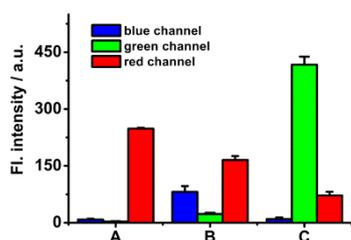
**Figure 6.** Detection of thiols and PAA in human blood serum (blue channel:  $\lambda_{em} = 467$  nm;  $\lambda_{ex} = 400$  nm; green channel:  $\lambda_{em} = 523$  nm;  $\lambda_{ex} = 466$  nm; red channel:  $\lambda_{em} = 598$  nm;  $\lambda_{ex} = 514$  nm). Sample A: probe **1** (5  $\mu\text{M}$ ); sample B: probe **1** (5  $\mu\text{M}$ ) treated with reduced serum (0.5 mL); sample C: probe **1** treated with reduced serum (0.5 mL), then further treated with NEM (1 mM).
