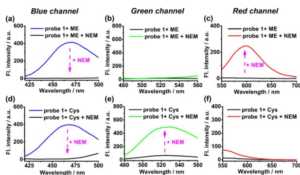
**Figure 4.** The fluorescence spectra of ME (240  $\mu\text{M}$ ) (a-c) and Cys (240  $\mu\text{M}$ ) (d-f) treated probe **1** (5  $\mu\text{M}$ ) upon further incubated with NEM (1 mM). Excitation at 400 nm for (a) and (d); 466 nm for (b) and (e); and 514 nm for (c) and (f).
