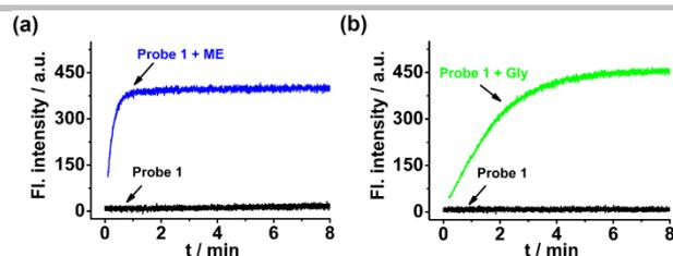
**Figure 3.** Time dependent fluorescence intensity changes of probe **1** (5  $\mu\text{M}$ ) in the absence and presence of (a) 300 $\mu\text{M}$  ME ( $\lambda_{\text{em}}$  = 467 nm;  $\lambda_{\text{ex}}$  = 400 nm) and (b) 300 $\mu\text{M}$  Gly ( $\lambda_{\text{em}}$  = 523 nm;  $\lambda_{\text{ex}}$  = 466 nm).
