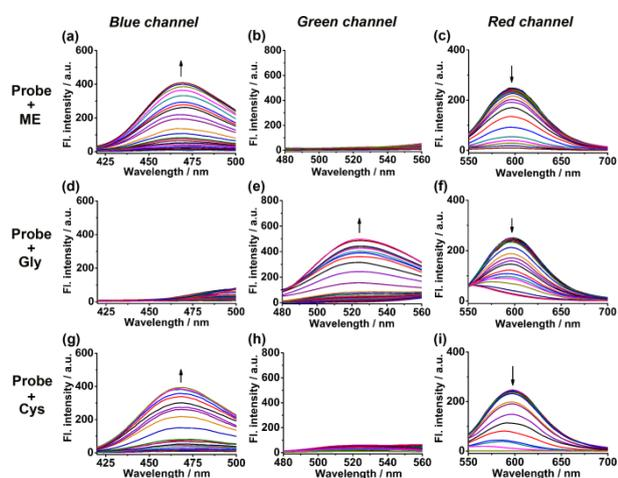
**Figure 2.** The fluorescence spectra of probe **1** (5  $\mu\text{M}$ ) upon addition of (a-c) ME (0-240  $\mu\text{M}$ ), (d-f) Gly (0-300  $\mu\text{M}$ ), and (g-i) Cys (0-240 $\mu\text{M}$ ) in 20 mM potassium phosphate buffer / DMF (v/v 1 : 3, pH 7.4) solution. Excitation at 400 nm for the (a), (d), and (g); 466 nm for (b), (e), and (h); and 514 nm for (c), (f), and (i).
