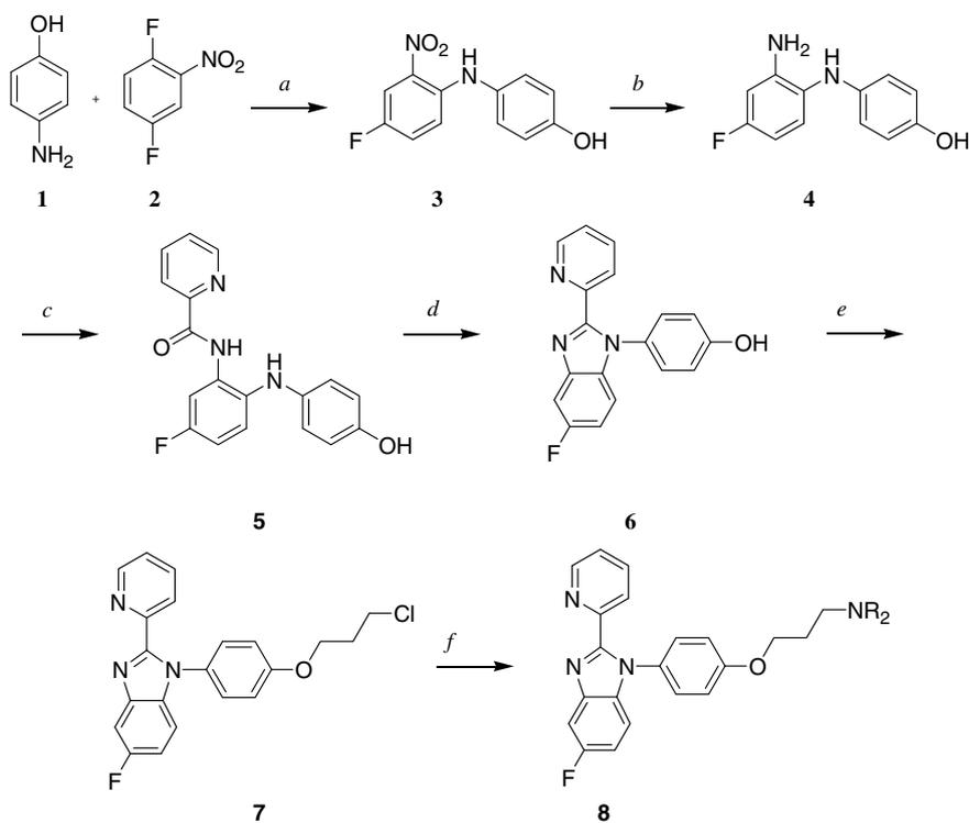
**Scheme 1.** Reagents and conditions: (a) Dioxane, reflux, 64%; (b) Ra-Ni, H<sub>2</sub>, MeOH, 83%; (c) picolinic acid, DCC, HOBT, CH<sub>2</sub>Cl<sub>2</sub>, 48%; (d) Acetic acid, 120 °C, 100%; (e) 1-bromo-3-chloropropane, K<sub>2</sub>CO<sub>3</sub>, acetone, reflux, 93%; (f) R<sub>2</sub>NH, CH<sub>3</sub>CN, *i*-Pr<sub>2</sub>NEt, 80 °C, 12–98%.
