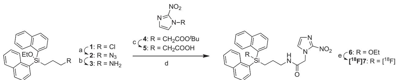
**Scheme 1.** Reagents and conditions: (a)  $\text{NaN}_3$ , DMF, reflux (88%); (b)  $\text{H}_2$ , 10% Pd/C, EtOH, 25 °C (73%); (c)  $\text{K}_2\text{CO}_3$ ,  $\text{CH}_3\text{CN}$ , reflux (98%); (d) EDCl,  $\text{NEt}_3$ ,  $\text{CH}_2\text{Cl}_2$ , 25 °C (63%); (e)  $\text{K}^{18}\text{F}$ /Krytoxif K2.2.2, AcOH,  $\text{CH}_3\text{CN}$ , 70 °C.
