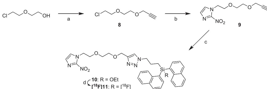
**Scheme 2.** Reagents and conditions: (a) NaH, THF,  $-78$  °C then  $\text{BrCH}_2\text{C}\equiv\text{CH}$ , reflux (94%); (b) 2-nitroimidazole,  $\text{K}_2\text{CO}_3$ , NaI, DMF, reflux (60%); (c) **2**,  $\text{CuSO}_4\cdot 5\text{H}_2\text{O}$ , sodium ascorbate, dioxane, 25 °C (44%); (d)  $\text{K}^{18}\text{F}$ /Krytoxif K2.2.2, AcOH,  $\text{CH}_3\text{CN}$ , 70 °C.
