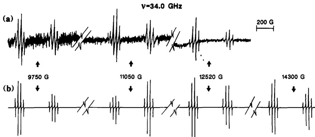
Figure 2. (a) EPR spectrum at Q-band of  $^{63}\text{CuPF}_3$  in adamantane at 100 K and (b) the simulated spectrum of  $^{63}\text{CuPF}_3$  produced from the parameters given in the text.
