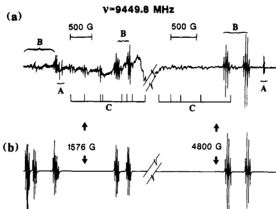
**Figure 1.** (a) EPR spectrum at X-band given by  $^{63}\text{Cu}$  atoms and  $\text{PF}_3$  codeposited into adamantane at 77 K and (b) the simulated spectrum of  $^{63}\text{CuPF}_3$  at X-band produced from the parameters given in the text.
