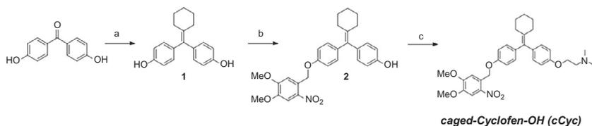
**Scheme 1** Improved synthesis of the caged cyclofen-OH **cCyc**. (a) cyclohexanone,  $\text{TiCl}_4$ , Zn, THF, reflux, 2 h (yield: 81–85%); (b) 4,5-dimethoxy-2-nitrobenzyl bromide,  $\text{K}_2\text{CO}_3$ , acetonitrile/ $\text{H}_2\text{O}$ , r.t., 16 h; (c) 2-(dimethylamino)ethyl chloride hydrochloride,  $\text{Cs}_2\text{CO}_3$ , acetone, reflux, 18 h (yield: 70%).
