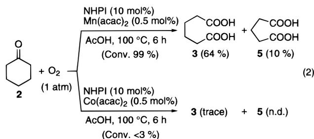
NHPI/Co(acac)<sub>2</sub> and NHPI/Co(acac)<sub>3</sub> systems, most of the starting **2** was recovered unchanged (eq 2). In contrast, the same oxidation of **2** by Co(acac)<sub>2</sub> in the absence of NHPI gave 61% of **3** in 92% conversion (eq 3).
