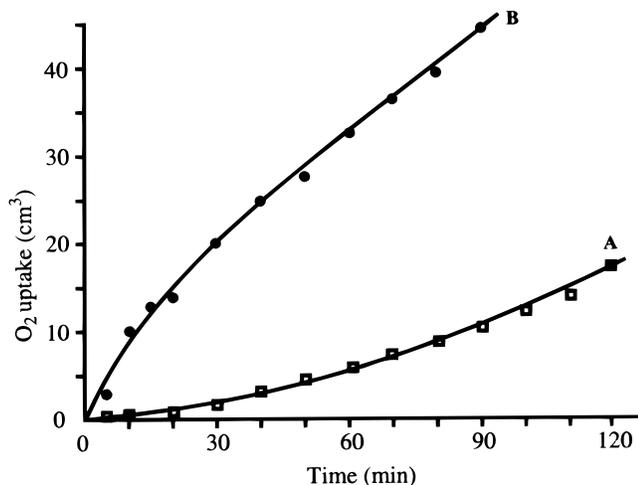
**Figure 2.** O<sub>2</sub> uptakes for the oxidation of cyclohexane (1) under atmospheric pressure of oxygen by catalytic systems. Conditions: cyclohexane 1 was allowed to react with oxygen (1 atm) in acetic acid (25 mL) at 80 °C in the presence of (A) NHPI (10 mol %) and Mn(acac)<sub>2</sub> (1 mol %), (B) NHPI (10 mol %), Mn(acac)<sub>2</sub> (1 mol %), and Co(OAc)<sub>2</sub> (0.1 mol %).
