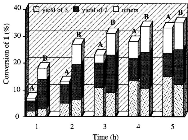
**Figure 1.** Time dependence for the oxidation of cyclohexane (1) to cyclohexanone (2) and adipic acid (3) by NHPI/Mn(II) (A) and NHPI/Co(II) (B) system in acetic acid at 100 °C. Conditions: cyclohexane 1 (3 mmol) was allowed to react with oxygen (1 atm) in acetic acid (7.5 mL) at 100 °C in the presence of NHPI (10 mol %) and metal salt (0.5 mol %).
