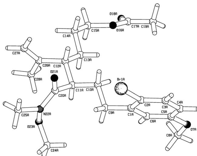
Figure 5. X-ray structure of Weinreb amide **13b** (only selected hydrogens are shown).
