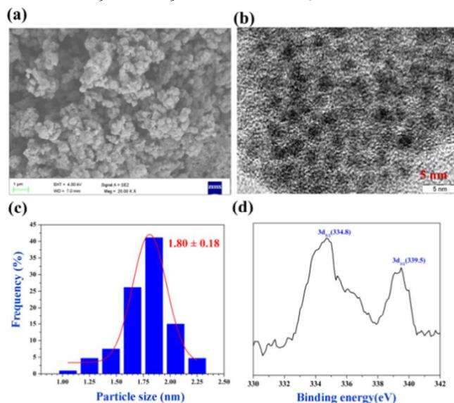
**Figure 3.** (a) SEM, (b) TEM, (c) particle size distribution and (d) XPS spectra of **Pd@CC1<sup>r</sup>**.
