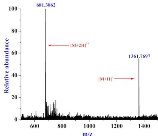
**Figure 2.** ESI-HRMS spectrum of  $CC1^f$  recorded in  $CHCl_3$ - $CH_3CN$  (1:1; v/v).
