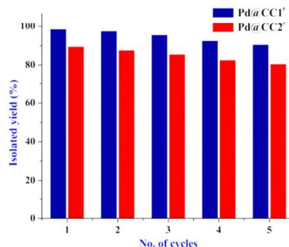
**Figure 4:** Recyclability of the  $\text{Pd@cage}$  catalysts.
