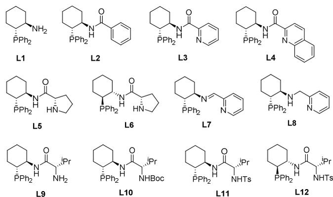
**Figure 1.** The structures of the chiral hexane-based P,N-ligands
