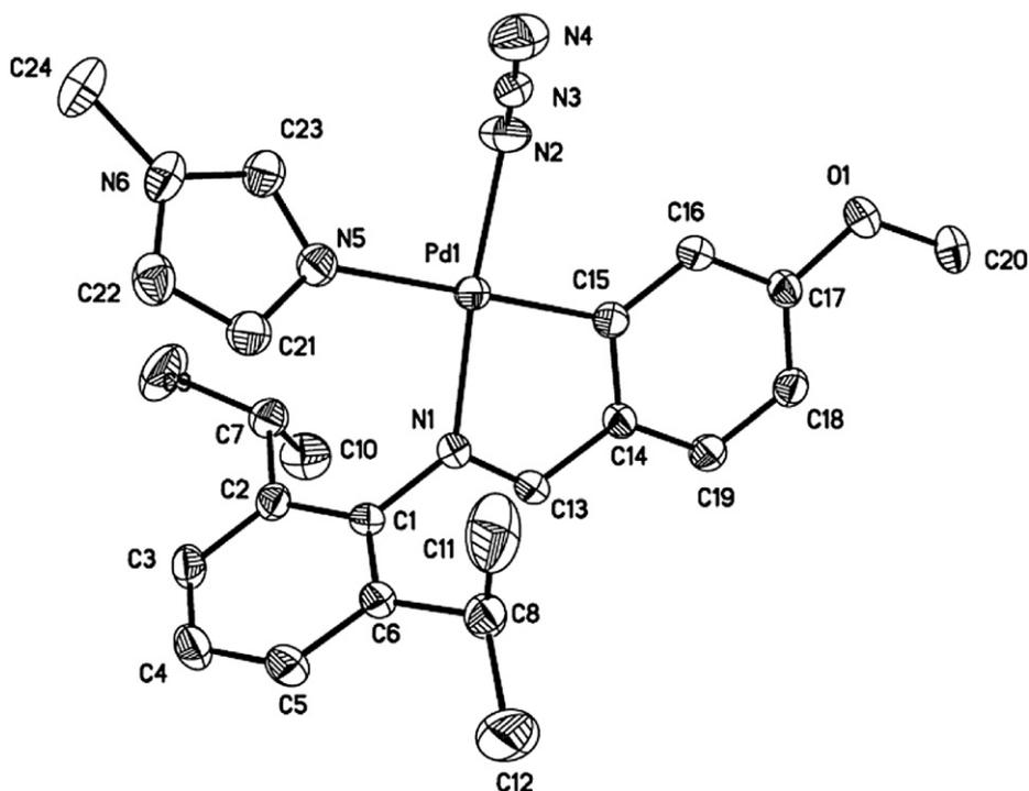
**Fig. 2.** Molecular structure of **6**. Selected bond lengths (Å) and angles (°): Pd1–C15 1.988(3), Pd1–N1 2.062(3), Pd1–N2 2.038(3), Pd1–N5 2.156(3), N2–N3 1.169(5), N3–N4 1.167(5); N1–Pd1–C15 80.67(12), N1–Pd1–N2 170.78(12), N5–Pd1–C15 178.79(12), N5–Pd1–N1 98.98(11), N3–N2–Pd1 120.0(3), C15–Pd1–N2 91.62(14), N4–N3–N2 176.0(4).
