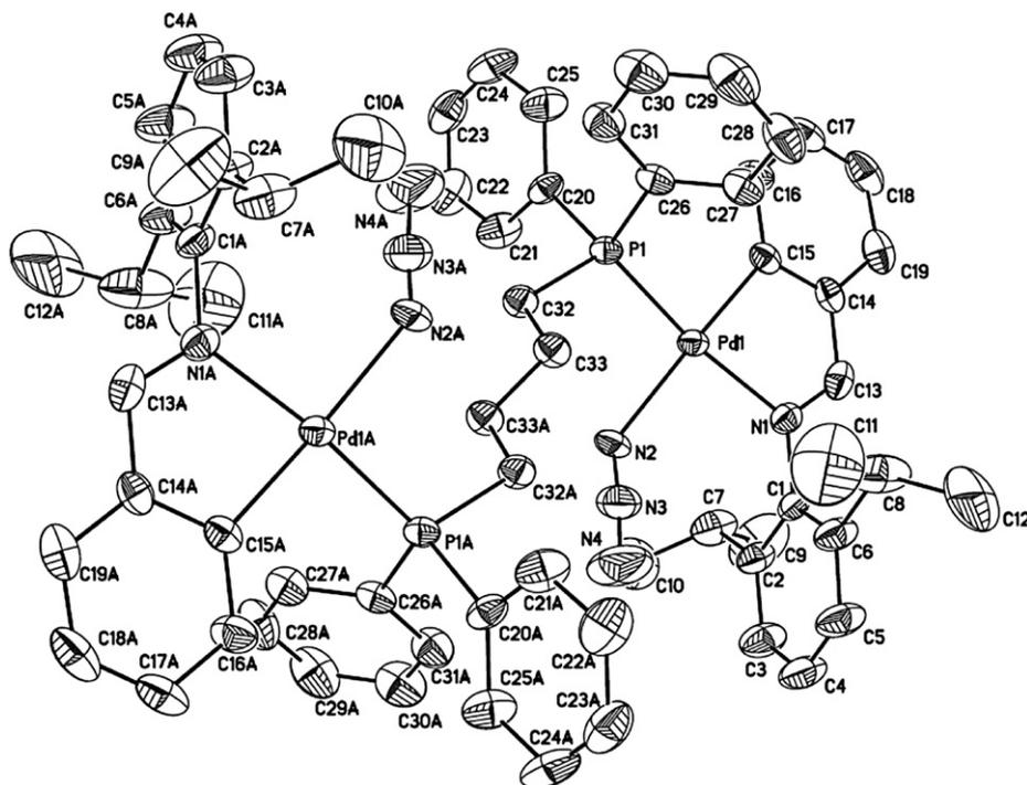
**Fig. 6.** Molecular structure of **17**. Selected bond lengths (Å) and angles (°): Pd1–C15 2.028(4), Pd1–N1 2.093(4), Pd1–N2 2.122(4), Pd1–P1 2.2548(11), N2–N3 1.136(6), N3–N4 1.178(7); C15–Pd1–N1 80.71(16), C15–Pd1–N2 166.58(17), C15–Pd1–P1 95.52(13), N2–Pd1–P1 92.21(12), N1–Pd1–P1 170.21(10), N3–N2–Pd1 132.4(4), N2–N3–N4 175.6(8), C20–P1–Pd1 116.88(14), C26–P1–Pd1 114.72(16), C32–P1–Pd1 112.22(15), C1–N1–Pd1 124.7(3).
