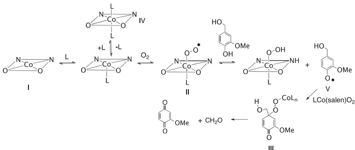
**Scheme 1.** Mechanism for *p*-quinone formation from *p*-substituted phenols catalyzed by **1**.
