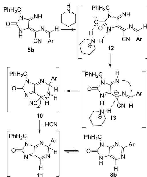
**Scheme 4.** Proposed mechanism for the formation of purine **8b** from 2-oximidazole **5b** in DMSO, in the presence of piperidine.
