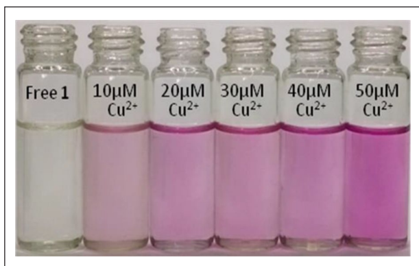
Figure 7. Visual colour change of \mathbf{1} ( 10 \mu\text{M} ) in 9:1 (v/v) THF-HEPES buffer solution (10 mM, pH=7.0) upon addition of 10–50 \mu\text{M} of \text{Cu}^{2+} ions.
