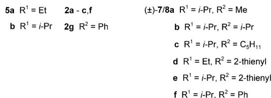
**Scheme 3.** Preparation of  $\beta$ -hydroxyphosphonates ( $\pm$ )-**8**. a) BuLi/THF,  $-78^\circ\text{C}$ ; b) AcOH; ( $\pm$ )-**8a**: 78%, ( $\pm$ )-**8b**: 88%, ( $\pm$ )-**8c**: 69%, ( $\pm$ )-**8d**: 91%, ( $\pm$ )-**8e**: 87%, ( $\pm$ )-**8f**: 92%.
