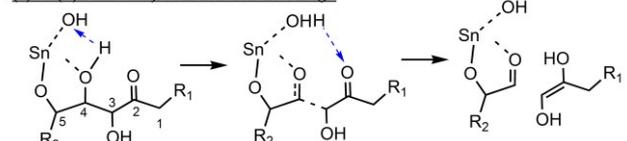
**Fig. 9** Proposed reaction paths based on theoretical computations for the isomerization and retro-aldol fragmentation.
