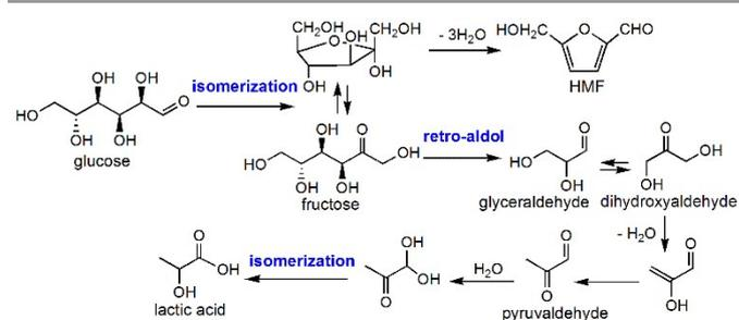
**Fig. 8** Reaction mechanism based on the DFT computations for the conversion of glucose to lactic acid in water.
