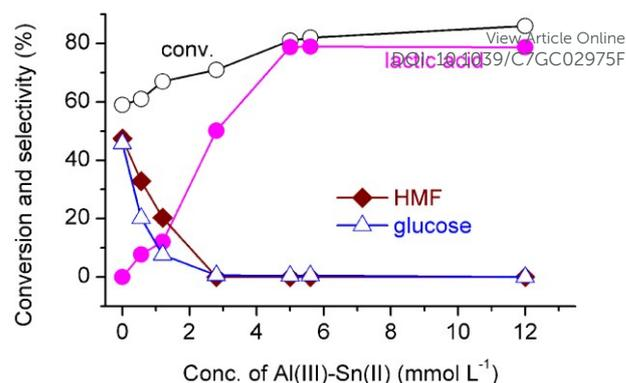
**Fig. 3** Effect of concentration of Al(III)-Sn(II) cations on catalytic behaviours for the conversion of cellulose. Reaction conditions: cellulose, 0.10 g (glucose unit, 0.62 mmol);  $\text{H}_2\text{O}$ , 20 mL;  $\text{N}_2$ , 3 MPa; 463 K; 2 h.  $\text{AlCl}_3$  and  $\text{SnCl}_2$  were used. The molar ratio of Al(III)/Sn(II) was 1/1.
