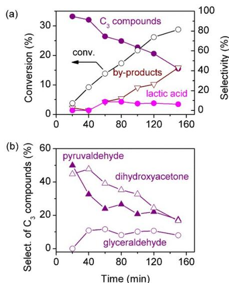
**Fig. 7** Conversion of fructose in the presence of Sn(II) cation. (a) Conversion and product selectivity. (b) Selectivity of C<sub>3</sub> compounds. Reaction conditions: fructose, 0.10 g (0.56 mmol); Sn(II), 0.10 mmol; H<sub>2</sub>O, 30 mL; N<sub>2</sub>, 3 MPa; 383 K. SnCl<sub>2</sub> was used. The selectivity of by-products, which mainly included polymeric compounds and humins, were calculated by subtraction of the selectivity of known products with 100%.
