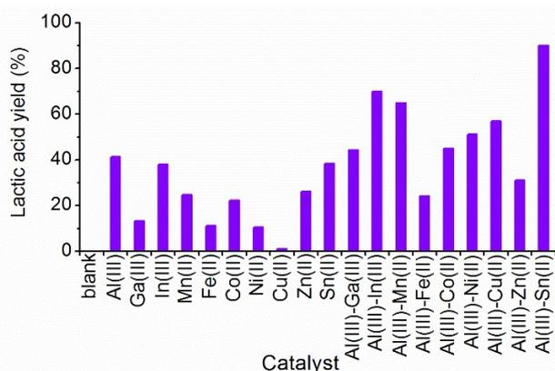
**Fig. 1** Catalytic conversion of fructose into lactic acid catalysed by various single cations or dual-cation combinations. Reaction conditions: fructose, 0.56 mmol; single or dual cations, 0.10 mmol; H<sub>2</sub>O, 20 mL; N<sub>2</sub>, 3 MPa; 463 K; 2 h. For dual cations, the molar ratio of the two components was 1/1.
