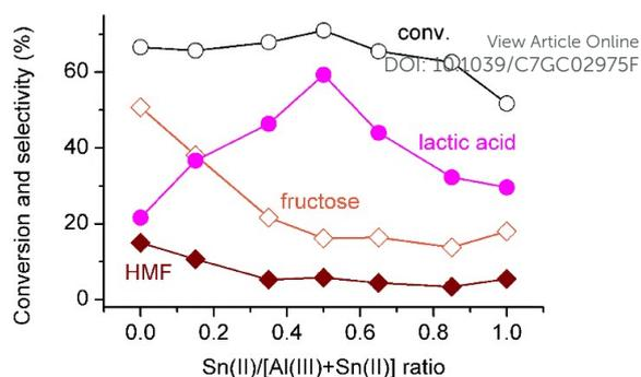
**Fig. 6** Effect of Al(III)/Sn(II) molar ratio on catalytic performances for the conversion of glucose. Reaction conditions: glucose, 0.10 g (0.56 mmol); H<sub>2</sub>O, 30 mL; N<sub>2</sub>, 3 MPa; 423 K; 0.5 h. AlCl<sub>3</sub> and SnCl<sub>2</sub> were used. The total amount of Al(III) and Sn(II) was fixed at 0.10 mmol.
