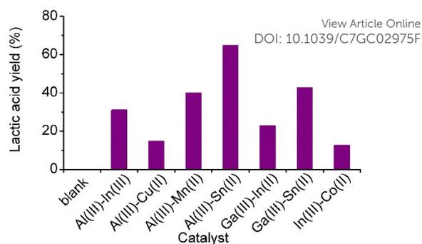
**Fig. 2** Catalytic conversion of cellulose catalysed by dual cations. Reaction conditions: cellulose, 0.10 g (glucose unit, 0.62 mmol); dual-metal cations (ratio = 1/1), 0.10 mmol; H<sub>2</sub>O, 20 mL; N<sub>2</sub>, 3 MPa; 463 K; 2 h.
