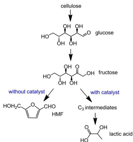
**Fig. 5** Reaction pathways for the conversion of cellulose in the presence and absence of Al(III)-Sn(II) catalyst.
