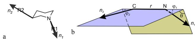
**Figure 4.** (a) Definition of vectors  $n_1$  and  $n_2$  (1,3-disubstituted piperidine scaffold used as an example). (b) Definition of geometric parameters  $r$ ,  $\varphi_1$ ,  $\varphi_2$ , and  $\theta$ .
