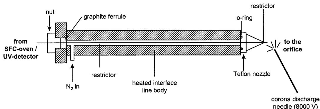
Figure 2. SFC/MS interface. The eluent is passed through the UV detector into the restrictor. The restrictor is held in place by the graphite ferrule in the back of the interface. Nitrogen is fed into the resistively heated interface, flowing out coaxially to the restrictor through the Teflon nozzle, which is placed just above the corona discharge needle.
