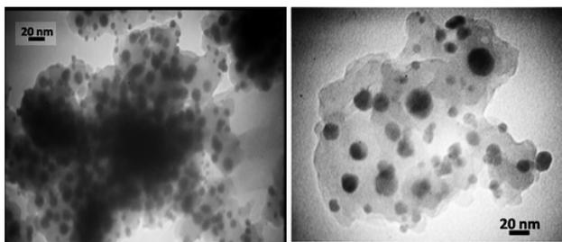
Fig. 4. TEM images of biosynthesized CuO NPs.
