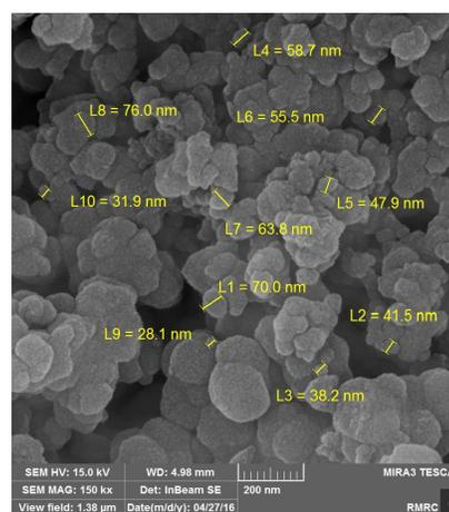
Fig. 2. FESEM image of biosynthesized CuO NPs.
