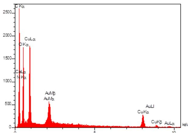
Fig. 3. EDX spectrum of biosynthesized CuO NPs.
