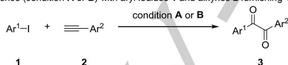
condition **A**: 2 mol% Pd(PPh<sub>3</sub>)<sub>4</sub>, 4 mol% CuI, NEt<sub>3</sub> (1.1 eq.), 1,4-dioxane, rt, 10 min
