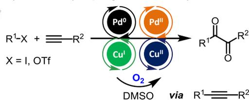
**Scheme 1.** Synthesis of 1,2-diketones from internal alkynes as starting material respectively intermediate.
