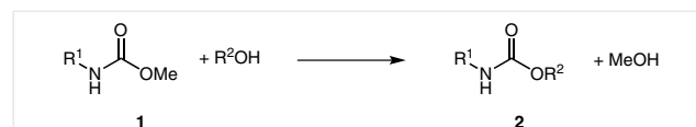
Scheme 1 Transcarbamoylation reaction of a urethane ( R^1 = aliphatic or aromatic group and R^2 = aliphatic group)
