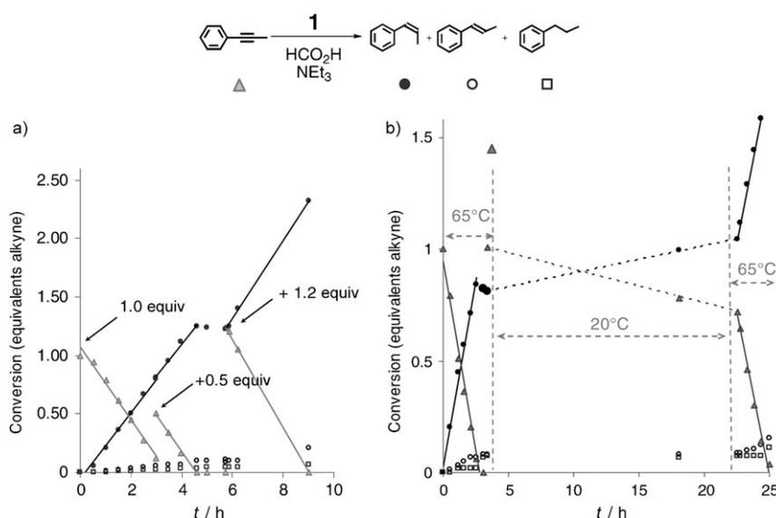
**Figure 1.** a) Transfer hydrogenation of 1-phenyl-1-propyne in THF, catalyzed by **1**, after adding subsequent equivalents: product distribution vs. time. b) Transfer hydrogenation of 1-phenyl-1-propyne in THF after adding one additional equivalent prior to stirring overnight at 20 °C: product distribution versus time.
