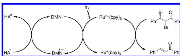
vic-Dibromo-,  $\alpha$ -halo-, or  $\alpha,\alpha$ -dibromocarbonyl compounds can be efficiently dehalogenated using catalytic tris(2,2'-bipyridyl)ruthenium dichloride ( $\text{Ru}(\text{bpy})_3\text{Cl}_2$ ) in combination with 1,5-dimethoxynaphthalene (DMN) and ascorbate as sacrificial electron donor. For this process, a visible light promoted photocatalytic cycle is proposed that involves the reduction of carbon halogen bonds via free radical intermediates.
