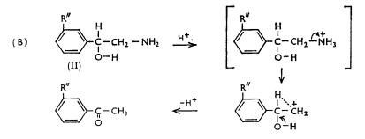
It seems that hydramine fission in presence of hydrochloric acid involves a unimolecular reaction and the formation of an 'onium ion; its kinetics are being studied. The reaction with  $\beta$ -hydroxyphenethylamine gave, unexpectedly, 1,3-diphenylcyclobutadiene; the predecessor of this was acetophenone which was isolated as its 2,4-dinitrophenylhydrazone when dinitrophenylhydrazine was added to reaction mixture.
