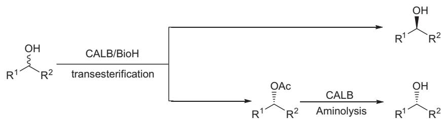
**Scheme 1.** General scheme of tandem and fully enzymatic procedure for the green resolution of a chiral alcohol.
