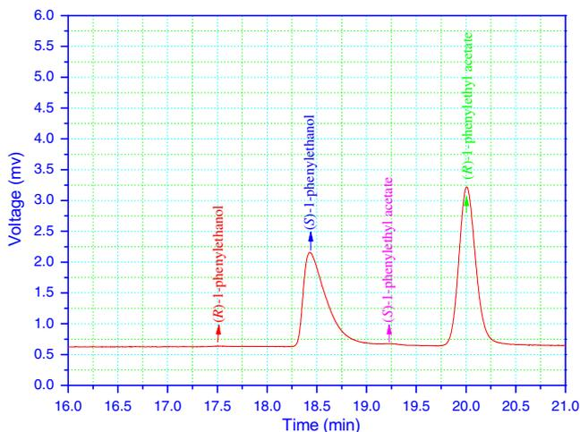
Figure 2. Chromatogram of the nearly-ideal resolution of (R,S)-1-phenylethanol.
