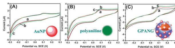
**Fig. 3** Cyclic voltammograms of the developed immunoassays toward 1.0 ng mL<sup>−1</sup> HIgG in (a) pH 8.0 NaBH<sub>4</sub>-PBS, (b) pH 8.0 NaBH<sub>4</sub>-PBS + 10 mM AP, and (c) pH 8.0 NaBH<sub>4</sub>-PBS + 10 mM NP by using various bionanotags: (A) AuNP-labelled Ab<sub>2</sub> antibodies, (B) PAN-labelled Ab<sub>2</sub> antibodies, and (C) GPANG-labelled Ab<sub>2</sub> antibodies. Scanning rate: 50 mV s<sup>−1</sup>.
