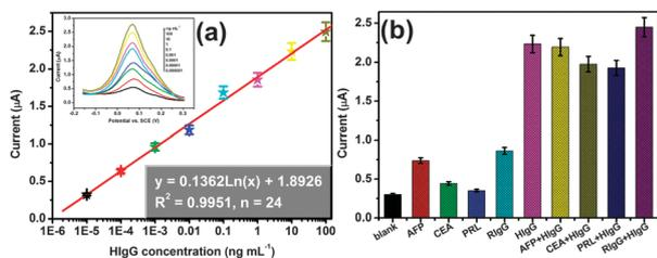
**Fig. 4** (a) Calibration plots and (b) specificity of the electrochemical immunoassay toward HIgG standards in pH 8.0 NaBH<sub>4</sub>-PBS containing 10.0 mM NP (inset: the corresponding DPV curves).
