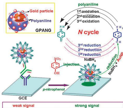
**Fig. 1** Schematic illustration of Au(III)-promoted polyaniline gold nanospheres with electrocatalytic recycling of self-produced reactants for signal amplification.
