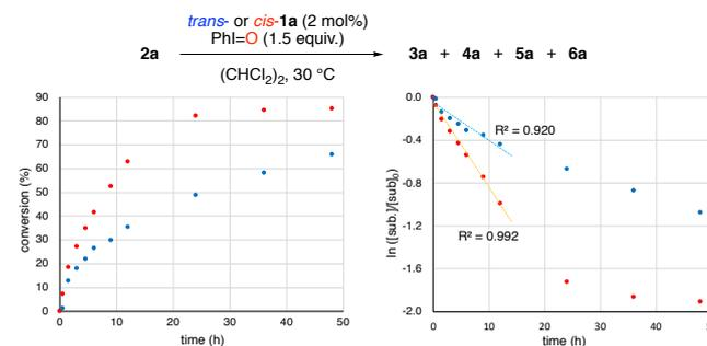
Figure 2. Monitoring *trans*-**1a** and *cis*-**1a**-catalyzed C–H hydroxylation of adamantane **2a**.
