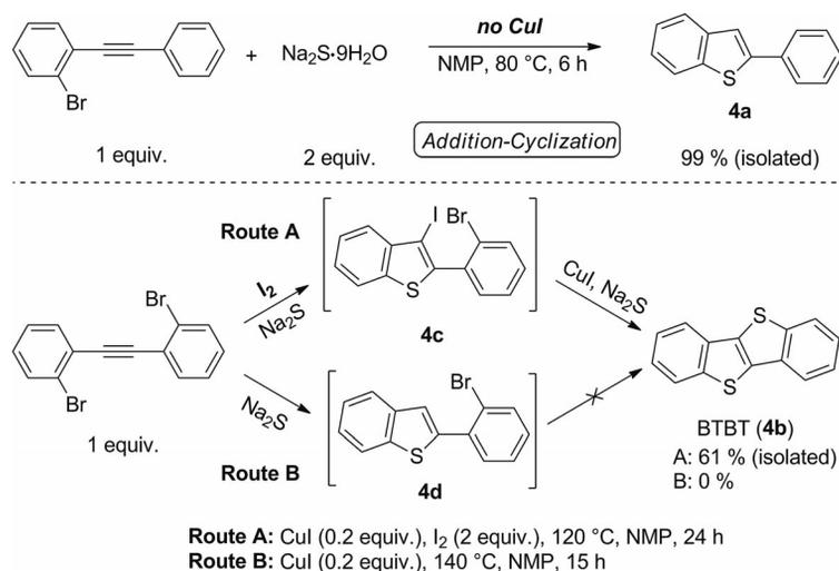
Scheme 2. One-pot syntheses of a BT derivative and of BTBT with  $\text{Na}_2\text{S}\cdot 9\text{H}_2\text{O}$  as sulfur source.
