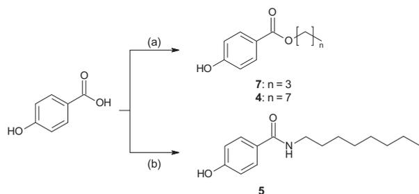
**Scheme 2.** Reagents and conditions of preparation of compounds **4**, **5** and **7**. (a) 1-butanol or 1-octanol, H<sub>2</sub>SO<sub>4</sub> (cat.), toluene, overnight; (b) SOCl<sub>2</sub>, triethylamine, toluene, 60 °C, 2 h, then 1-octylamine, overnight.
