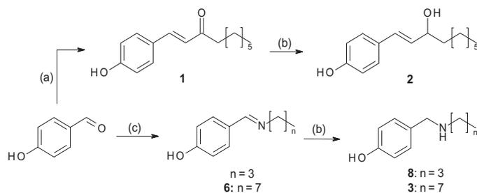
**Scheme 1.** Reagents and conditions of preparation of compounds **1–3**, **6** and **8**. (a) 2-nonanone, NaOH 40%, overnight; (b) STAB, AcOH, 4 h; (c) butylamine or octylamine, THF, 60 °C, 1 h.
