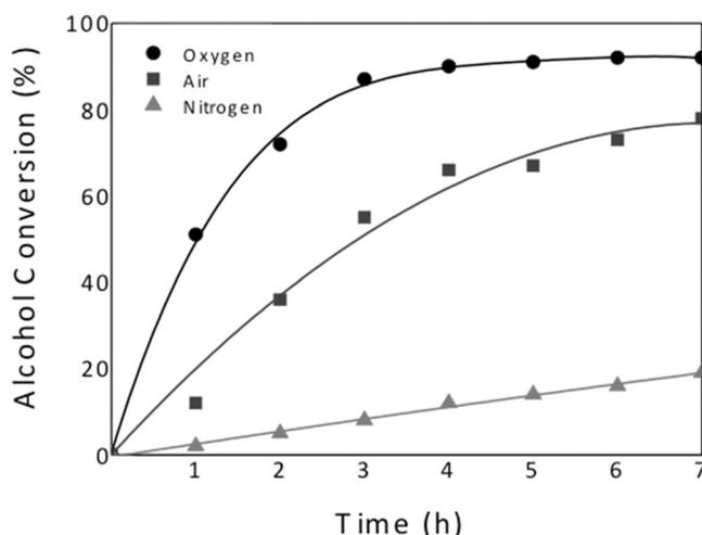
**Figure 3.** Conversion of 1-phenylethanol with **SBA-15-Thia** as a function of the time under oxygen, air or nitrogen atmosphere.
