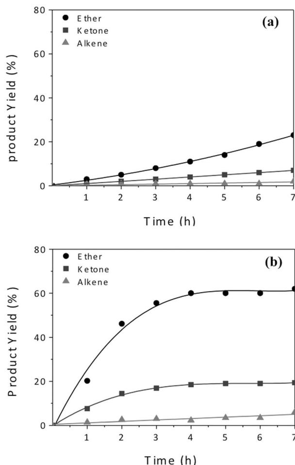
**Figure 6.** Kinetic profile of the reaction of 1-phenylethanol catalyzed by **Homo-Thia-Me** under an air (a) and an oxygen (b) atmosphere.
