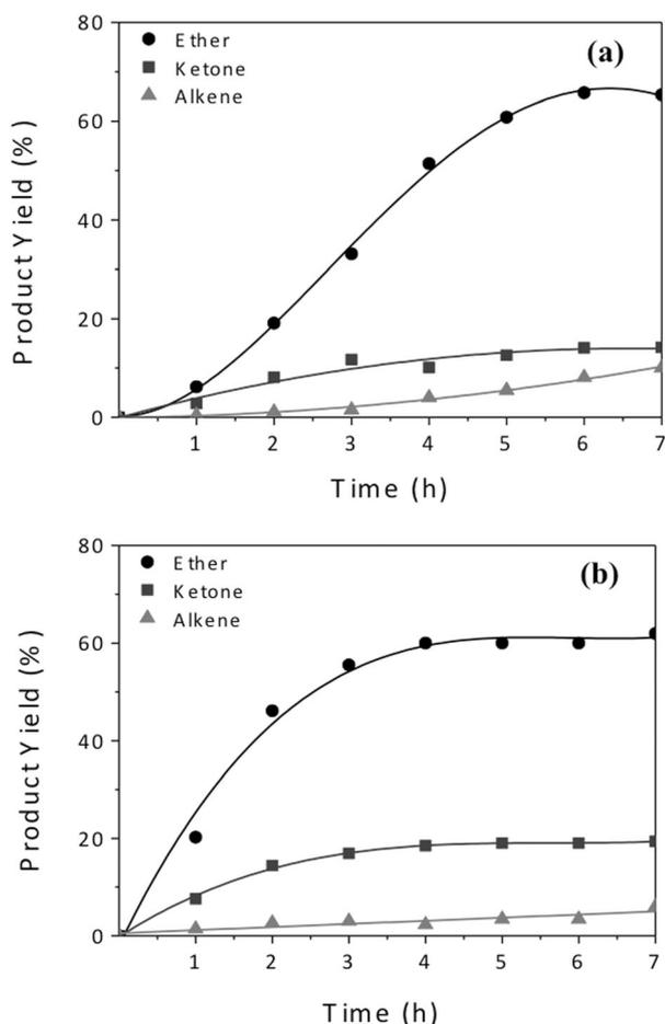
**Figure 5.** Kinetic profile of the reaction of 1-phenylethanol catalyzed by **Homo-Thia-H** under an air (a) and an oxygen (b) atmosphere.
