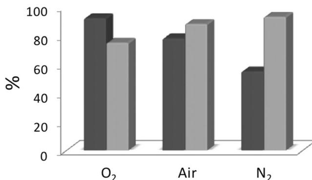
**Figure 2.** Conversion (dark grey) and selectivity (light grey) in the etherification reaction of 1-phenylethanol mediated by **SBA-15-Thia** after 7 h.
