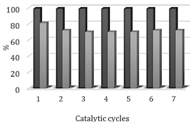
**Figure 8.** Conversion (dark grey) and selectivity (light grey) in multiple catalytic runs of the etherification reaction of 1-phenylethanol promoted by **SBA-15-Thia**.
