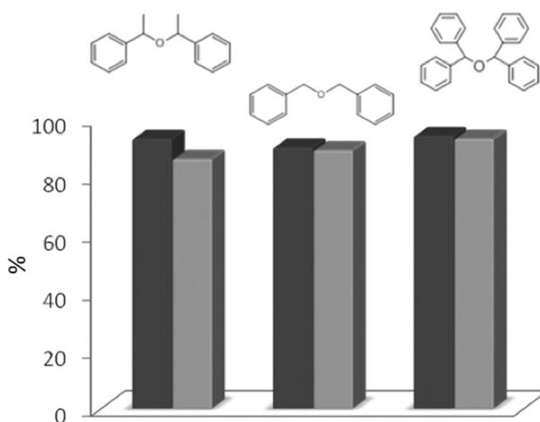
**Figure 9.** Conversion (dark grey) and selectivity (light grey) in the etherification reaction of 1-phenylethanol, benzyl alcohol and diphenylmethanol.
